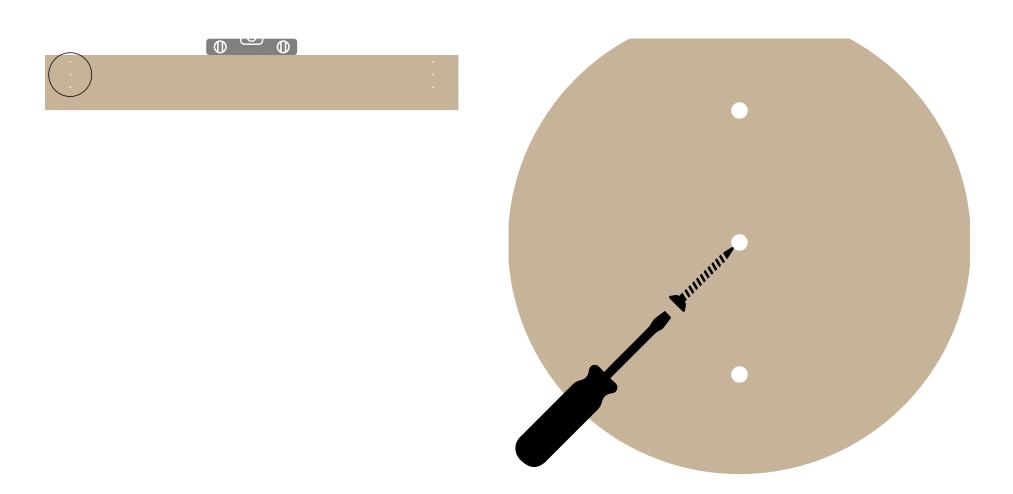
3A) Place wood on wall and make sure top edge is level 3B) Screw through center holes and into wall to hold board in place while hole locations are predrilled
