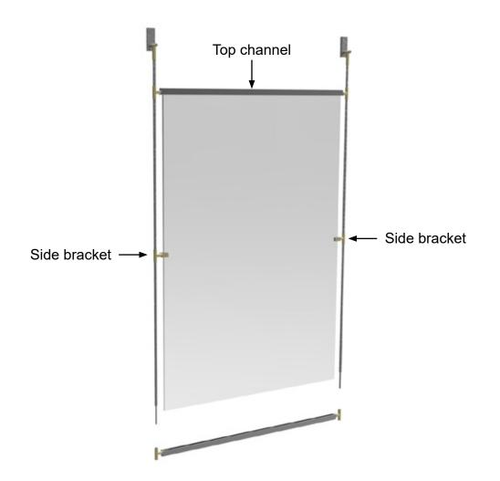
9a) Slide glass through side brackets and into top channel.9b) Slide bottom channel onto frame, fitting glass into channel
