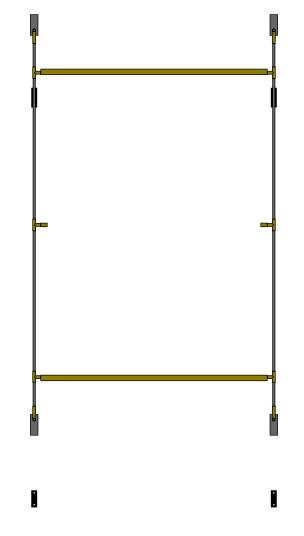
7a) Test installation recommended prior to installing glass7b) After confirming proper wall bracket installation,remove frame from wall brackets to install glass
