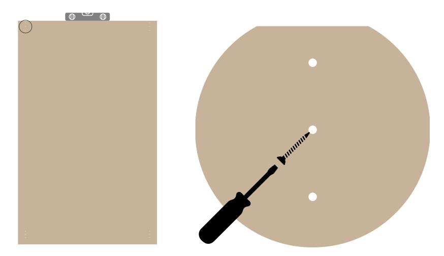
3A) Place wood on wall and make sure top edge is level3B) Screw through center holes and into wall to holdboard in place while hole locations are predrilled
