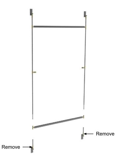
8a) Unscrew bottom two parts (twist counterclockwise) to remove8b) Mirror support will slide off frame
